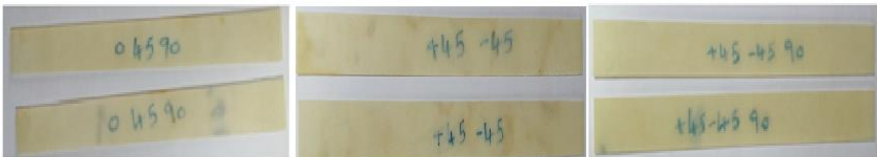
fig 1. Tensile specimen G16 (0°/45°/90°)
