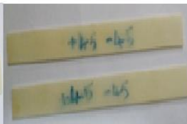
fig 7. Tensile specimen G4 (+45°/-45°) (+45°/-45°/90°)
